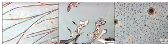
Figure 5. Optical microscopy images of the films of compounds 3a (left), 3b (middle), and 3c (right) drop-casted from THF on a plain SiO_2 silicon-wafer substrate.
